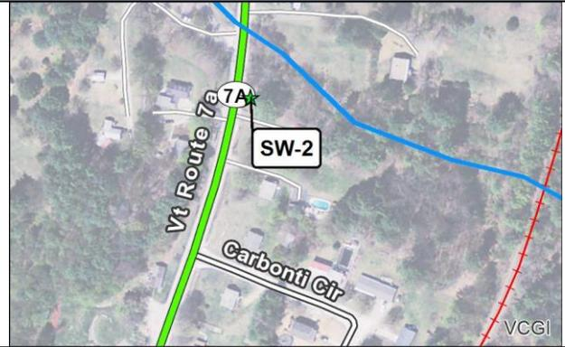
**Site Description:** Drainage ditches with runoff from Route 7A and adjacent residential areas drain north to a first-order stream (Photos 1 & 2). Significant gravel deposits settle out in the ditch just north of Carbonti Circle.
