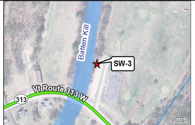
**Site Description:** Runoff from the gravel parking lot and a portion of Route 313 drains directly into the Batten Kill. Some erosion is present along the stream bank.
