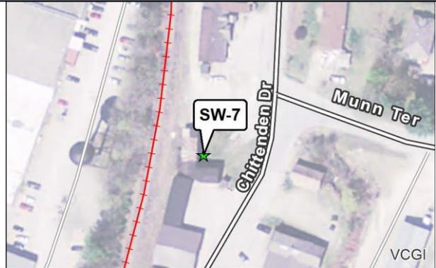
**Site Description:** Runoff from Chittenden Drive, Munn Terrace, and a parking area drains to a former loading dock for Miles Lumber Company (Photos 1 & 2). May be within the railroad ROW. Runoff enters a standpipe and is diverted directly into the underground stream.
