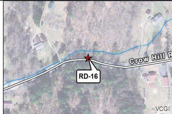
**Site Description:** This area has a severely eroded conveyance down a steep slope draining directly to the stream on the north side of the road (Photos 1 & 2). Rill erosion is present on the south side of the road due to shallow unstable drainage ditches. This road segment ranked 3<sup>rd</sup> (top 1%) in the water quality prioritization based on REI data.
